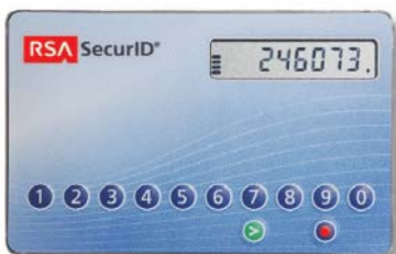
RSA SecurID SID900 Transaction Signing Authenticator. The PIN pad enables implementation of the digital signing function.
