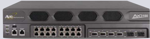
AX 3100: Enterprise/ISP 16 Gigabit Copper ports, 4 G SFP ports and 2 XFP 10 Gig ports.
